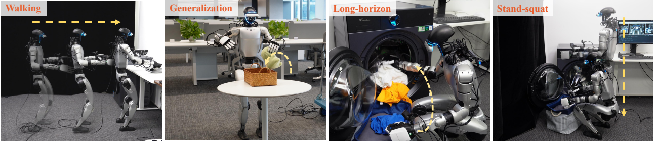
Figure 1. HumanoidExo , a wearable exoskeleton system that transfers human motion to whole-body humanoid data. HumanoidExo provides an efficient solution that bridges the embodiment gap between humans and robots, facilitating the collection of diverse datasets. We tested it on three real-world tasks, and the results show that it helps humanoid robots generalize to new environments, learn complex tasks from limited data, and acquire new skills like walking.
